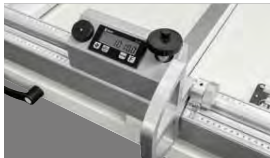
Electronic readouts on the squaring stops The stops can be easily read even from distance.
