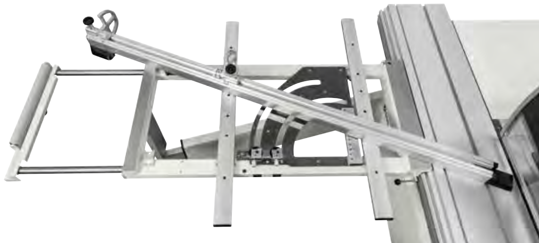
Squaring frame with "Compex" device with automatic self-adjustment of stops position in respect of the blade and rule tilting angle. Furthermore, thanks to the dedicated frame structure, it is possible to carry out tilted cuts keeping the squaring rule comfortably within the operator's reach , both in acute cuts and in obtuse ones, without renouncing to a valid support of the piece.
